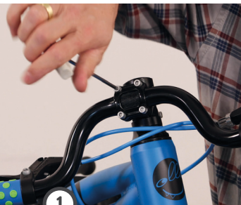
1 loosen the handlebar clamp
