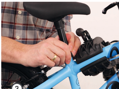
3 Tighten the saddle
