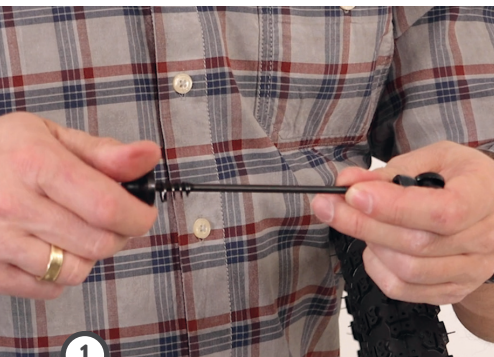
1 Open the quick-release axle
