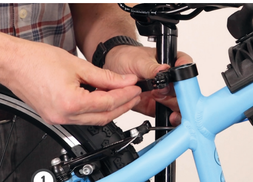
1 Release quick release skewer
