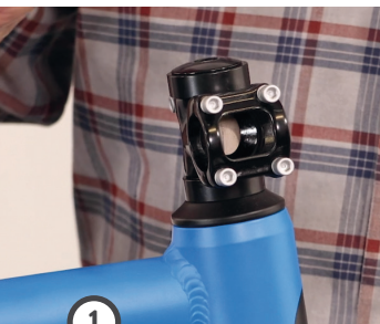
1 open handlebar clamp
